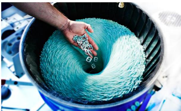
Intensive processing through different centrifugal forces
